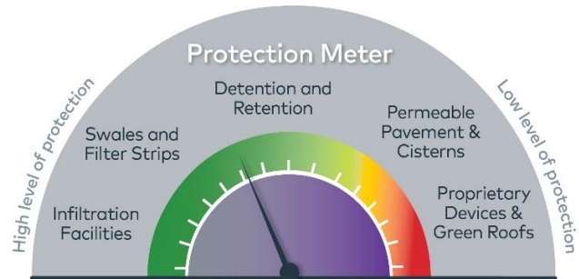
Figure 3-21. Stormwater BMP Protection Meter
