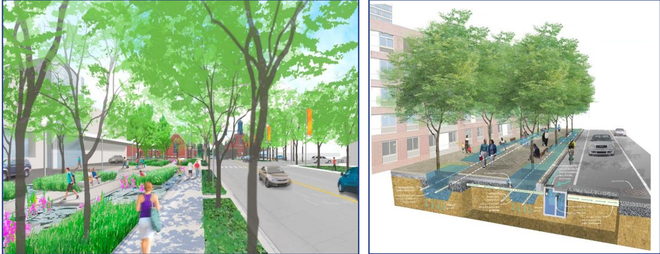
Left: Streetscape ground surface rendering. Right: Rendering of underground design shows street water is used to irrigate street trees. Also note the multi-modal features. Graphics source and designer: Sasaki Landscape Architects
