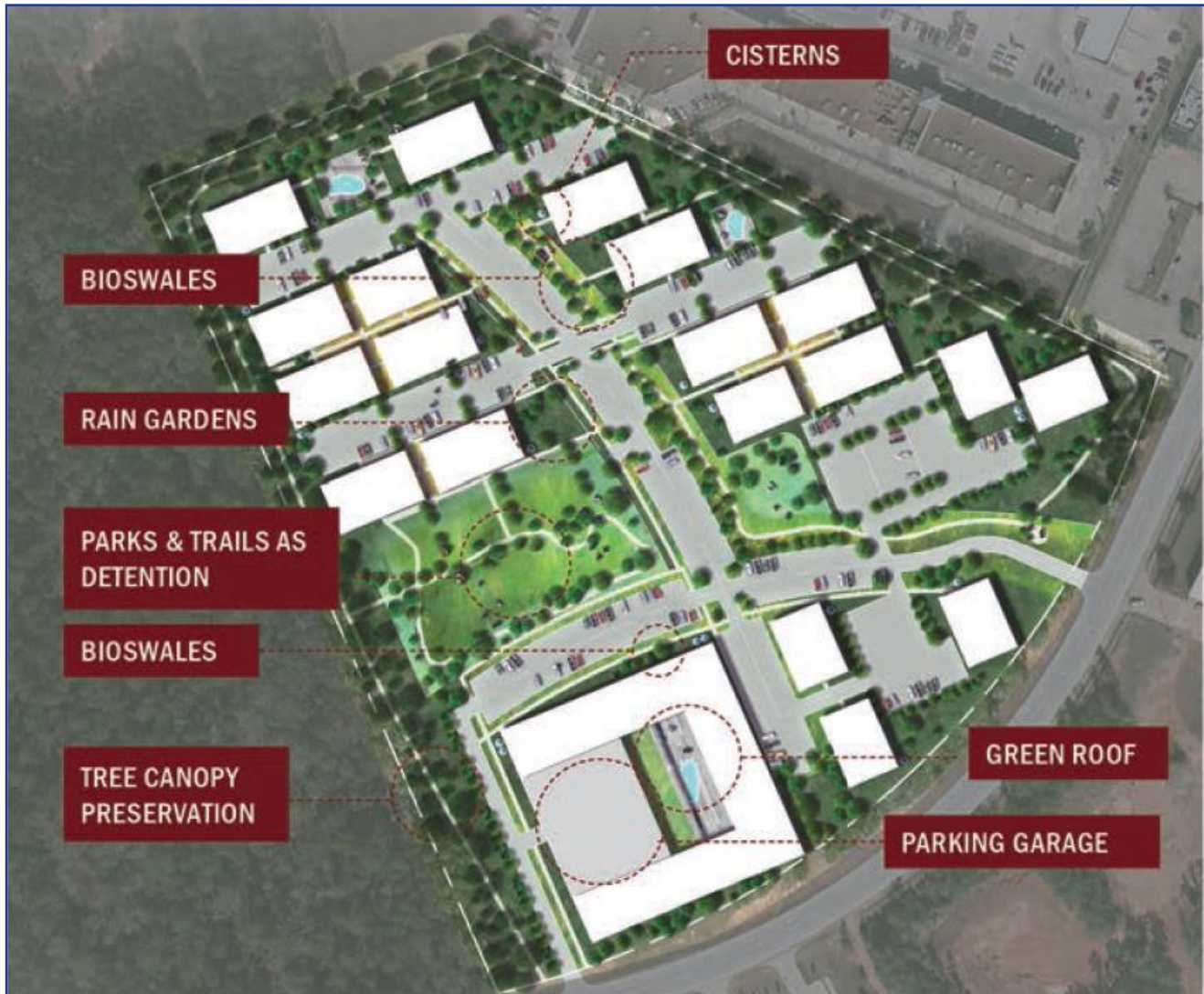
Figure 5-11. Example of a PUD with LID and GI-BMs (Source: Wood E&S, Inc.)
