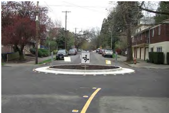
Example 2 Traffic calming device and pedestrian crossing on Buchanan and 24th
