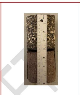
Photo #10: 4-inches asphalt, 4-inches brick
