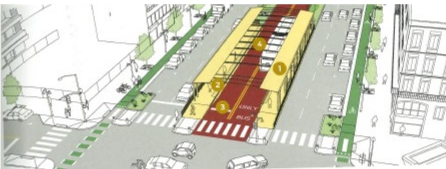
**Median or Center Lane Stop**, rather than being placed at the outermost lane of the roadway, this bus stop is provided in the center lane. Signal phasing and routes help enable this infrastructure type many times for Bus Rapid Transit service. Pedestrian access to these stops is provided by intersection or midblock pedestrian crossings.
