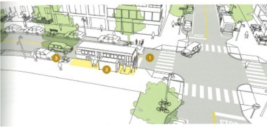
**Boarding Bulb out stop**, this bus stop projects out from curb and in line with parking or lane width to bring passengers out to the edge of the traffic lane with the traffic lane isn't adjacent to curbside.
