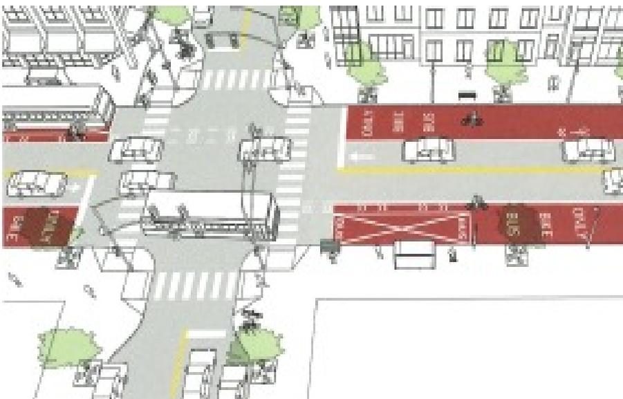
**Bus/Transit Lane based Bus Stop**, this bus infrastructure has exclusive access to this lane, rather than sharing it with other single occupant motor vehicle traffic.
