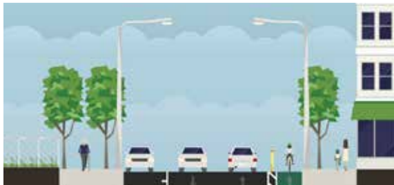
Local street design section Two-lane road with parking lane, bike lane, sidewalks
