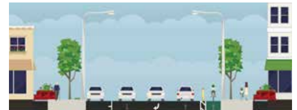
Arterial street design section (two-way, center-turn lane, parking lane, bike lane, landscaped sidewalks)
