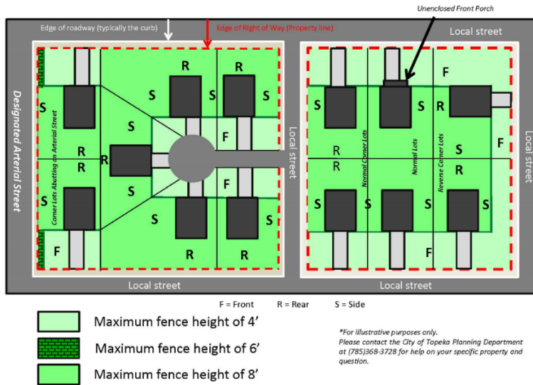
Fence Height Limit Diagram* (for "R" and "M" zoning districts)
