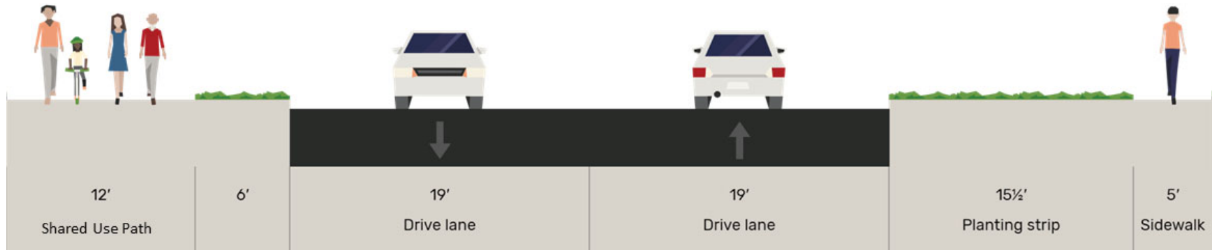
Figure 6. Section B (Adams St to Branner St) – Proposed (38' curb to curb) *
