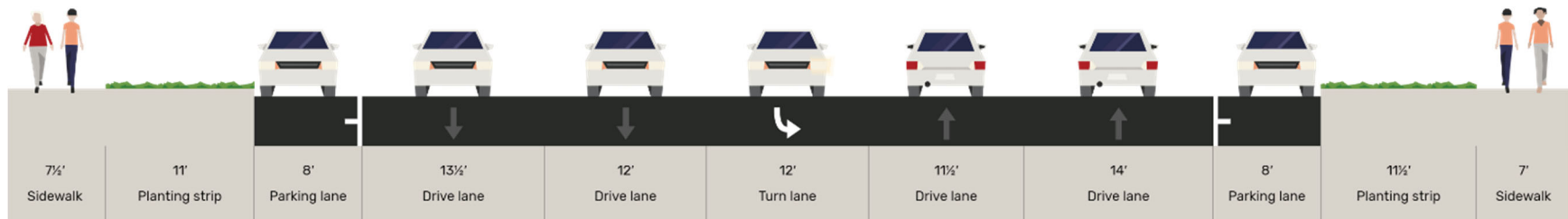
Figure 2. Section A (Kansas Ave to Adams St) – Existing (79' curb to curb)
